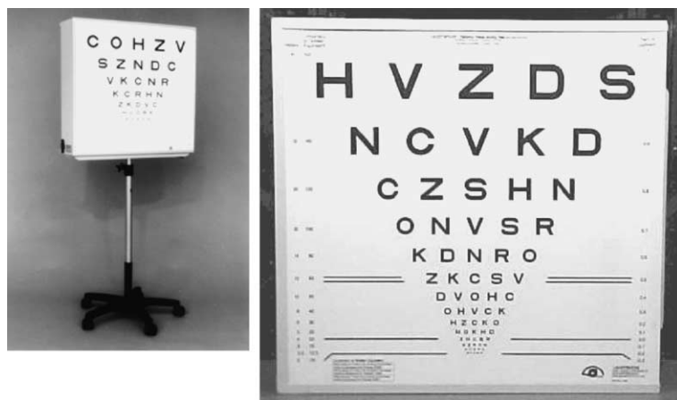
Fig. 1. Measuring visual acuity with the shown ETDRS reading chart represents the standard parameter to monitor visual acuity in AMD patients within clinical trials. Different charts are used for right and left eye. Results are expressed in lines and characters read by the patient.
